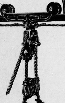
has fewest parts, greatest durability, holds load any elevation, does it automaticlly, and doesn't wear the ope, requires no trip block, as direct draft, uses only one-half as much rope, horses travel half as far, saving one-half the time. Let us show. Our price saves you
