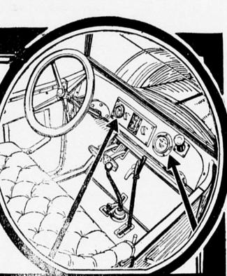
Speedometer, fuse box, ignition, lights, battery regulator, all mounted flush on instrument board.
