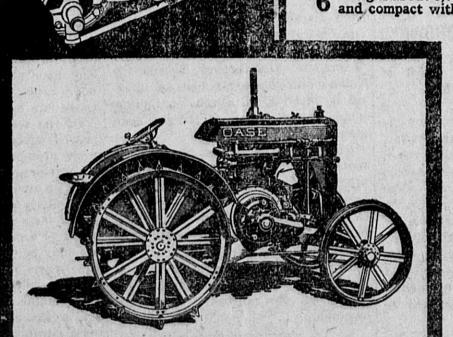
Rated 10 horsepower on drawbar, but develops nearly 14 horsepower. Rated 18 horsepower on the belt, but delivers about 24 horsepower. This insures abundant reserve
