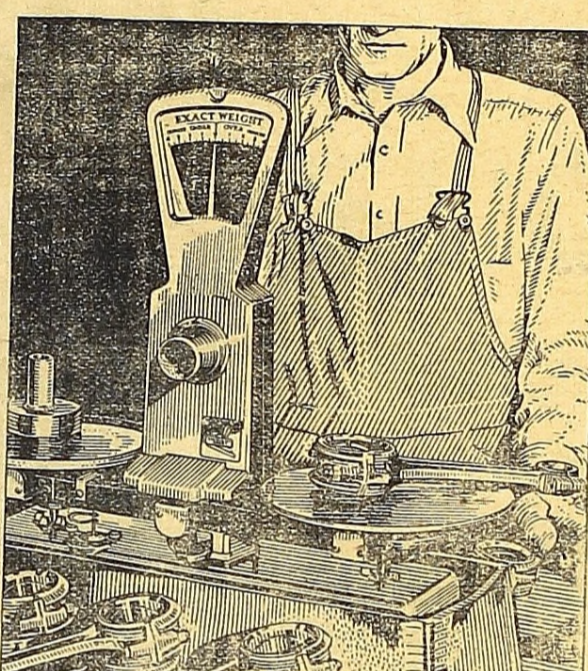
Chevrolet connecting rods are matched in sets of six to within one-quarter ounce, and are individually fitted by hand to the crankshaft. Bearings are of babbit metal cast into the rods under heavy air pressure and at 800 degrees Fahrenheit.
