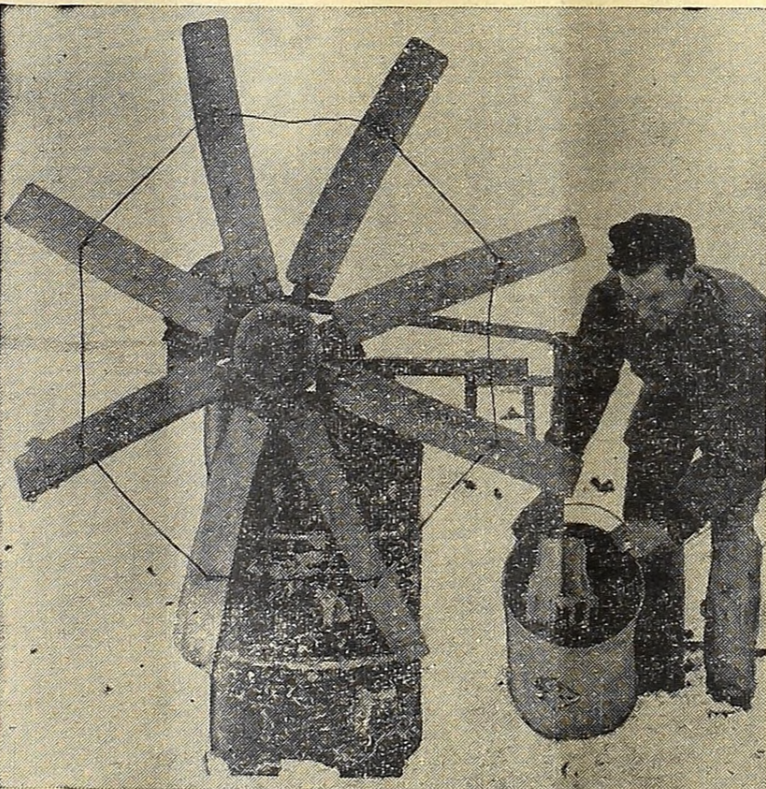
When the Aleutian winds blow we may or may not have snow, but at least Pvt. Early Krech of St. Paul, Minn., will have snow white laundry. He rigged up this windmill washing machine in which a chain and sprocket connected to the blades of the windmill delivers power to the wooden paddlewheels in the wash bucket.
