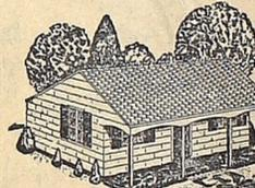
Complete information is provided for laying out guide lines, digging foundations and putting in footings. Framing and sheathing instructions are also included. Assembly illustrations show exact location of all framing members. After the sub-flooring is nailed to the floor joists, the four wall frames are built complete on the working platform. Each is then raised and nailed in position.
