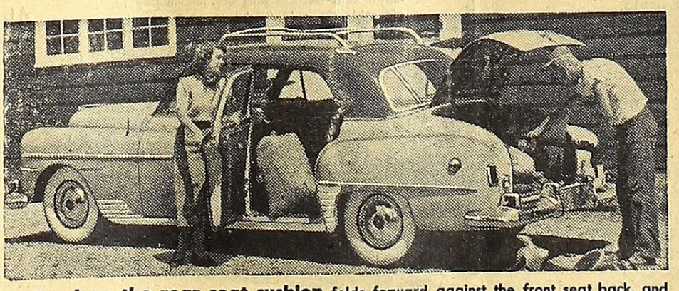
See how the rear seat cushion folds forward against the front seat back, and rear seat back turns down to form flat, level-loading platform. Spare tire can be carried in passenger compartment, or in well at right of luggage compartment.
