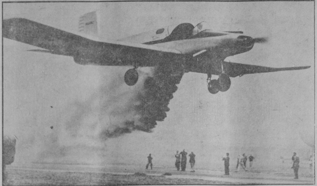
AERIAL FARMHAND—Swooping low to show off its crop-dusting ability, the "Fletcher Utility" goes through its paces at Rosemond, Calif. It is said by its manufacturers to be the first plane specifically designed for farm work to be put into volume production. Of all-metal construction, and with a 42-foot wingspan, the aerial workhorse is designed to pick up a 1250-pound load from an 870-foot, unimproved flight strip.
