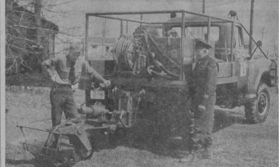
NEW FIRE FIGHTING EQUIPMENT—This new International four-wheel drive truck and pumper went into service in Isoco County last week. Owned and manned by the Michigan Department of Conservation, the truck is equipped with a hydraulic lift plow for cutting fire lines. It is operated from the cab or rear of the truck. Shown inspecting the new equipment is Fire Officer Bert MacGregor and Conservation Officer Arthur Leitze.—Tawas Herald Photo.
