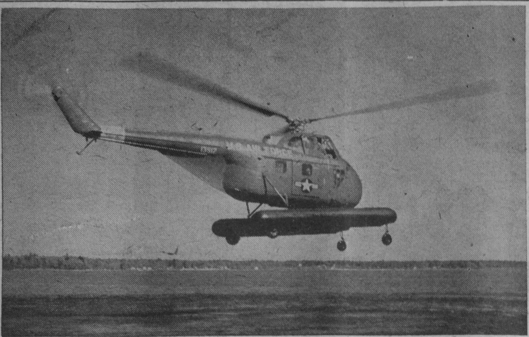
HERE IS ONE of the newest "whirlybirds" to go into service at Wurtsmith Air Force Base. It is equipped with pontoons to facilitate rescue of airmen who may go down in Lake Huron. It replaces the crash boats which were formerly stationed at the mouth of the AuSable River.
