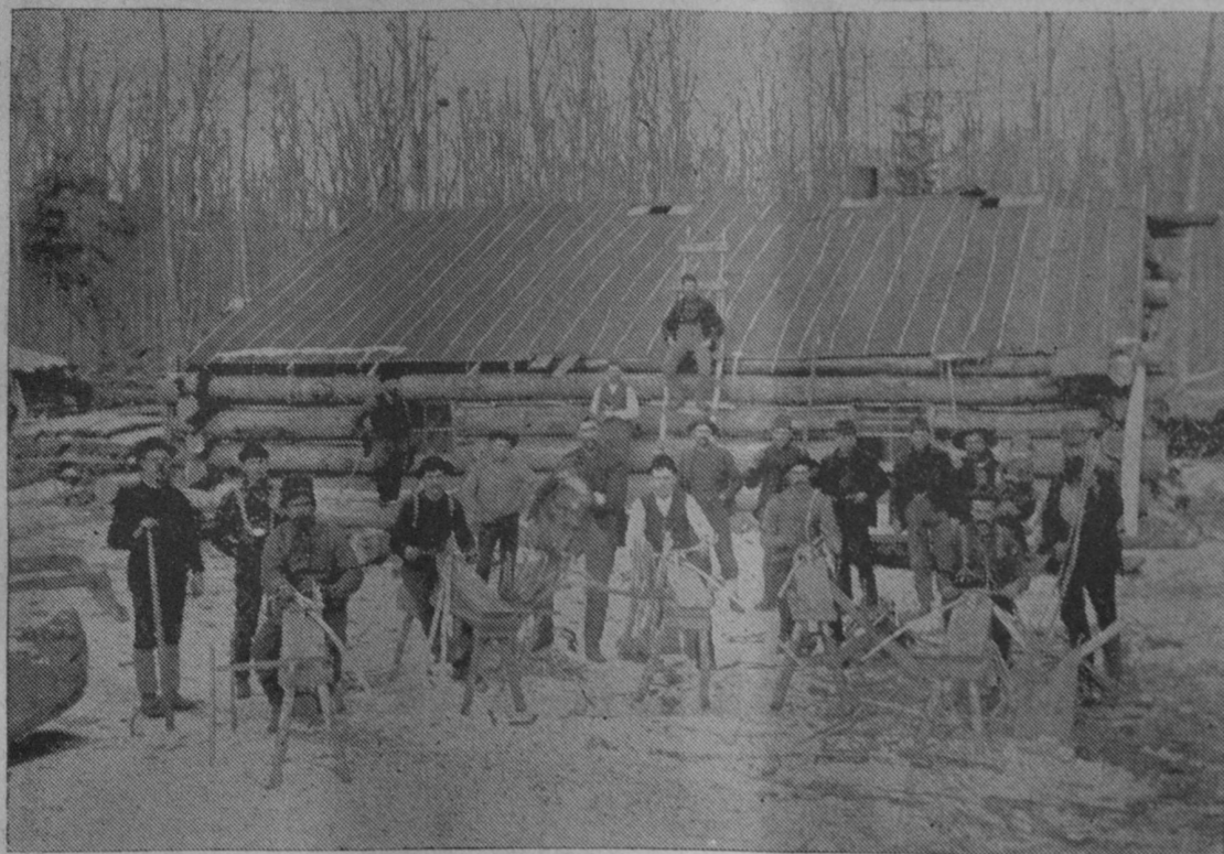
HOOP YARD owned by Matthias Schneider in Sherman Township in the 1870s. The men in the picture are splitting and shaving black and white ash from which the hoops were made.
