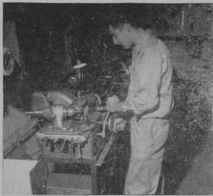
Ottawa Equipment Company's machine shop is modernly equipped and offers facilities for complete tune-up and engine rebuilding. Here, Donald Penman is resurfacing a valve using modern Sunnen equipment.
