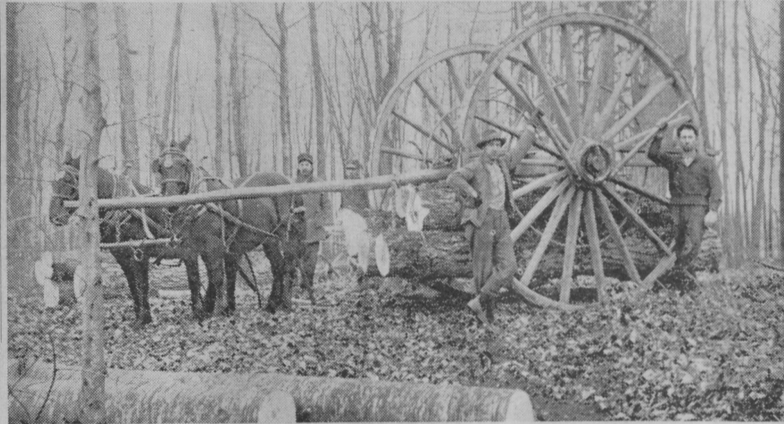
BIG WHEELS like these were used to haul logs out of the forest and into the AuSable River banking grounds. The husky lumberjacks in the foreground have fastened their cant hooks to the hub of the wheel. Hardwood logs are being moved here.—Joseph Barkman Collection.
