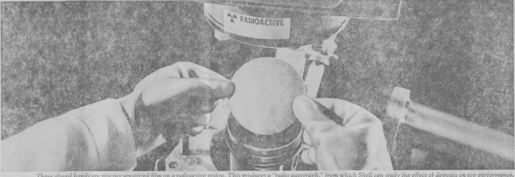
These gloved hands are placing sensitized film on a radioactive piston. This produces a "radio autograph," from which Shell can study the effect of deposits on top performance.
