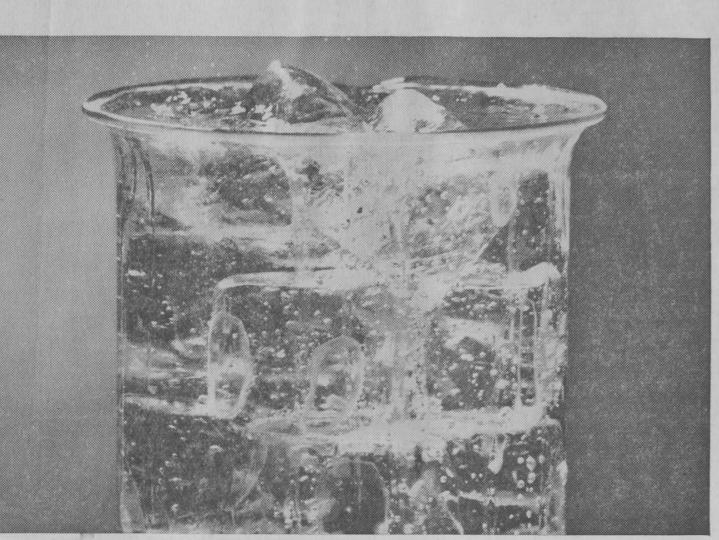
Butane boils and bubbles even though beaker is filled with ice cubes. It is rapidly turning into vapor-the way boiling water turns into steam. Butane's ability to vaporize at low temperatures helps Super Shell gasoline give you quick starts in cold weather.
