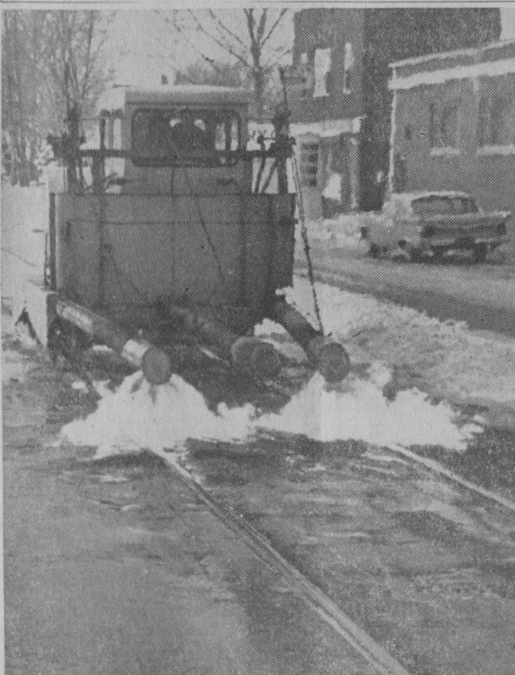
A NOVEL WAY to keep railroad tracks clear of ice was used by the Detroit and Mackinac Railway Company last week. This week-killing unit, normally used during warmer weather, was operated along the rails and flames spouting from the two booms on the front did the trick. It is shown here at the Newman Street intersection at East Tawas.—Tawas Herald Photo.
