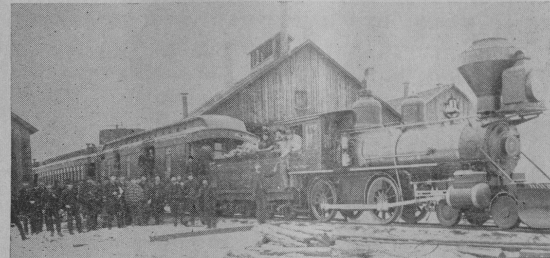
ONE OF THE Detroit, Bay City and Alpena Railway's track trains in the early 1880s, just after it had pulled into the yards at Tawas. Note the spark arrester on the stack which typified the wood burner.—Tawas Herald Collection.
