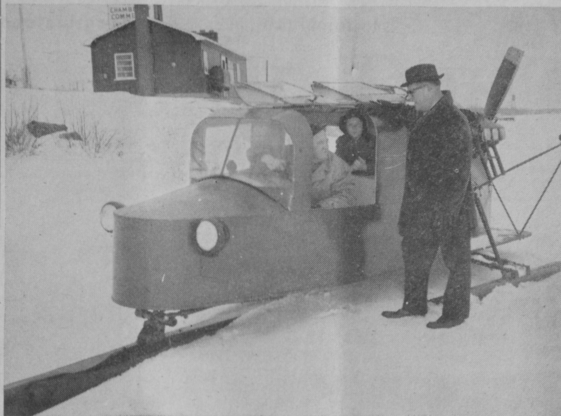
DAN THAYER, Hale area tree grower, has the perfect solution to winter driving problems— a special pusher-type propeller can reach a speed of 135 miles per hour. It seats six persons and weighs 1,200 pounds. Thayer has used the craft on Houghton and Higgins Lakes, along with Loon and AuSable Lakes in Iosco County.—Tawas Herald Photo.
