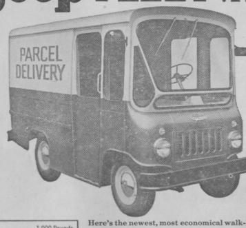
.....1,000 Pounds Engine. . Hurricane, 4 Cyl. F-Head, 72 hp. Overall Length Load Space Volume.....170 Cu. Ft. Interior Height Rear Load Area..... Load Area......62½ inches Length of Load Area.....87½ inches Interior Width Rear
