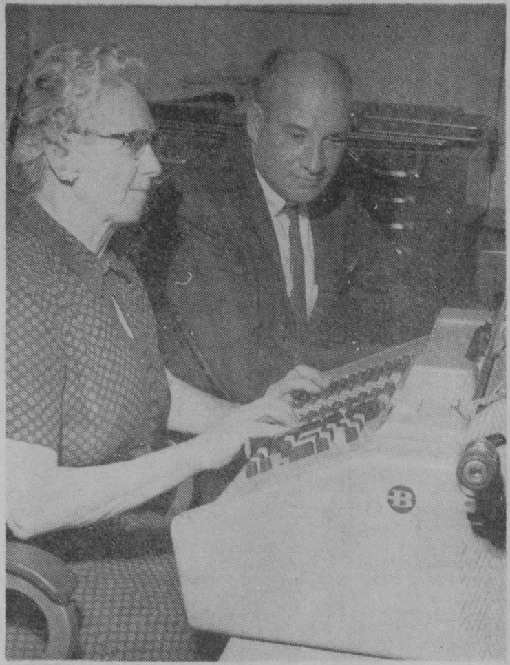
APPROVAL was given last week by the Iosco Board of Supervisors for purchase of a tax billing machine at a cost of $9,000. Shown operating the machine is Mrs. Harold Lundahl, manager of the county's tax billing department. Looking on is Henry Oates, chairman of the board of supervisors. This complicated machine prints valuations and individual totals on pages of tax rolls and also is used in preparation of tax statements. Oates said that the machine would complete preparation of tax rolls and statements in a matter of 22 days, while today, each supervisor spends about three weeks on such work. It is also expected to reduce the chance of error. Iosco now has one of the most modernly equipped tax billing departments of any comparable size county in the state.—Tawas Herald Photo.
