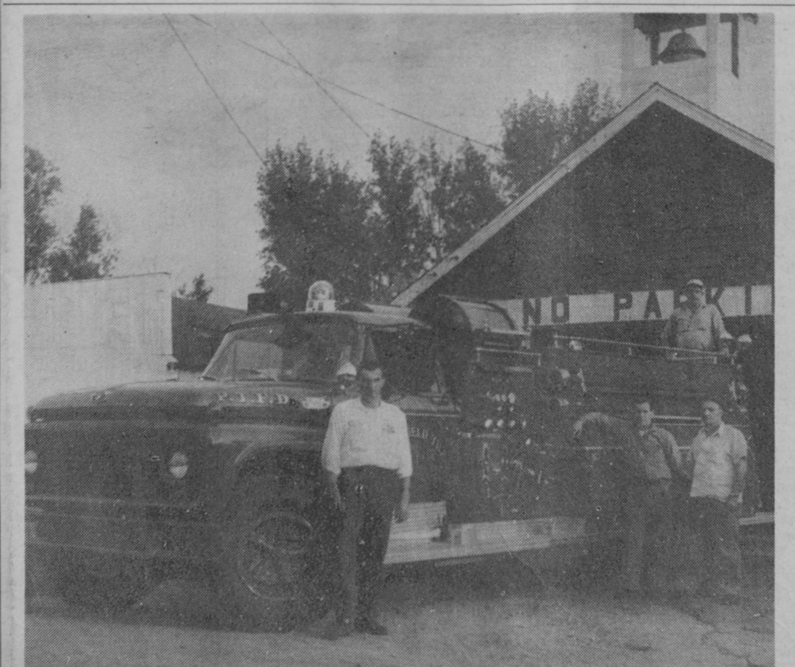
PLAINFIELD TOWNSHIP FIRE DEPARTMENT received delivery last week of its new $20,000 John Bean fire truck. Purchased as part of a $25,000 general obligation bond issue approved by voters, the truck is of the latest design. With a 750-gallon water supply tank, the truck is equipped with high pressure fog and volume pumps, heated hose beds, 1,400 feet of new hose, automatic rewinds. Six members of the department attended a two-day school at Lansing last week studying operation and maintenance of the new truck. Firemen in the picture from left are Assistant Chief Jack Slosser, James Schroeder and Lt. Lloyd Springsteen. George Spearman stands on the back. Work on the township's new fire hall is expected to be completed in about a month.—Tawas Herald Photo.
