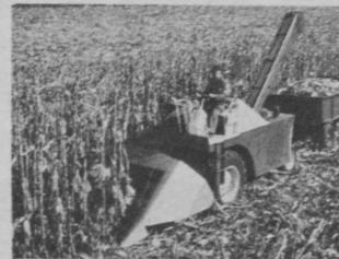
SUPERPICKER CORNHEAD designed for New Idea's new Uni-Picker, Uni-Shell, Uni-Combine, has patented snapping roll design, high-speed dual auger elevators for non-stop picking.
