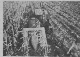
PULL-TYPE SUPERPICKERS. 1-row, 2-row for standard rows, 2-row for narrow rows. All 2-row pulls offer interchangeable husking beds, shellers, grinders.
