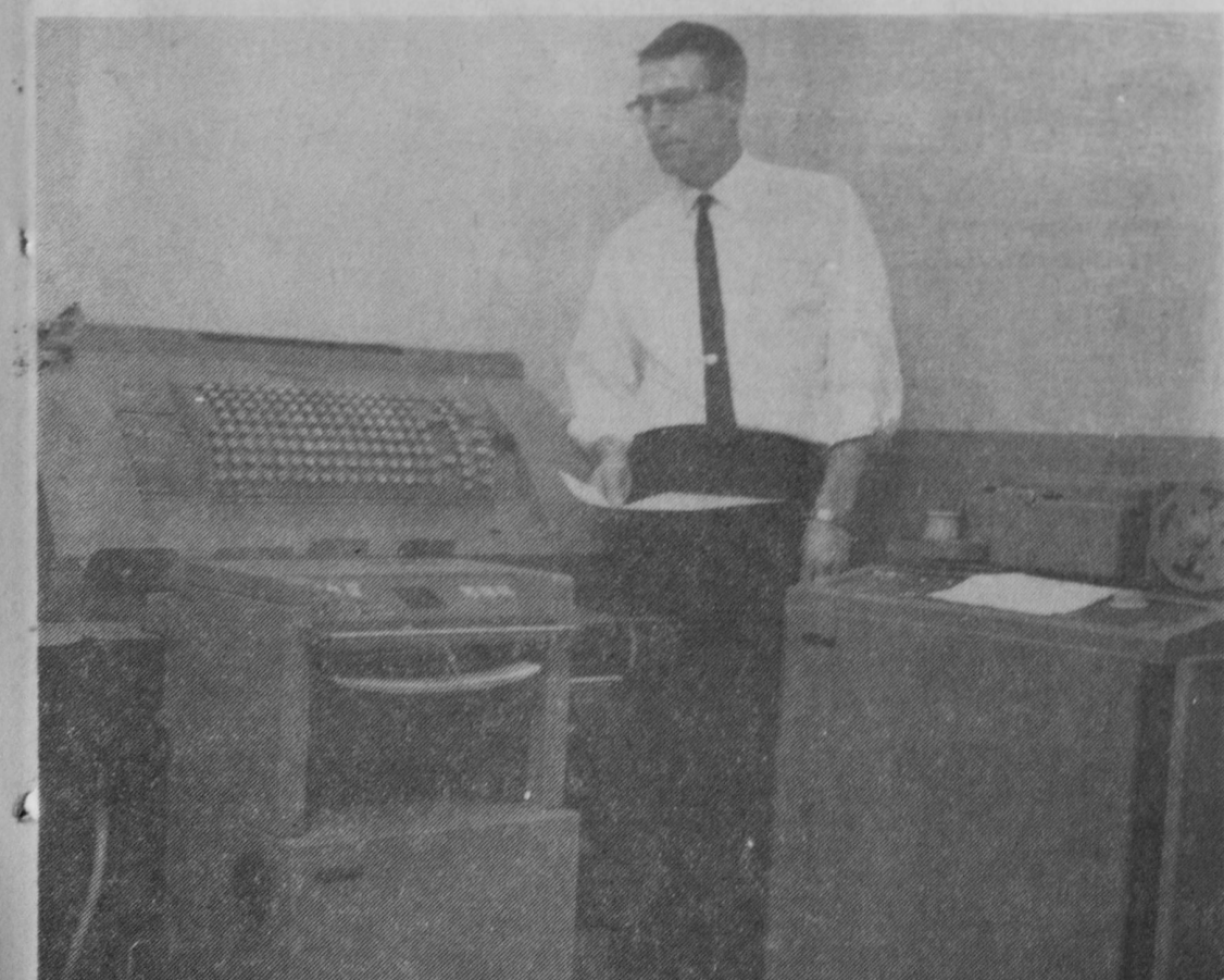
PEOPLES STATE BANK of East Tawas has received delivery on its completely automated Postronic machine, which goes into operation sometime early next year. Shown looking over the equipment is Richard Lee. The equipment is to be used for commercial ledger posting and is operated from a tape prepared by an IBM computing machine.—Tawas Herald Photo.
