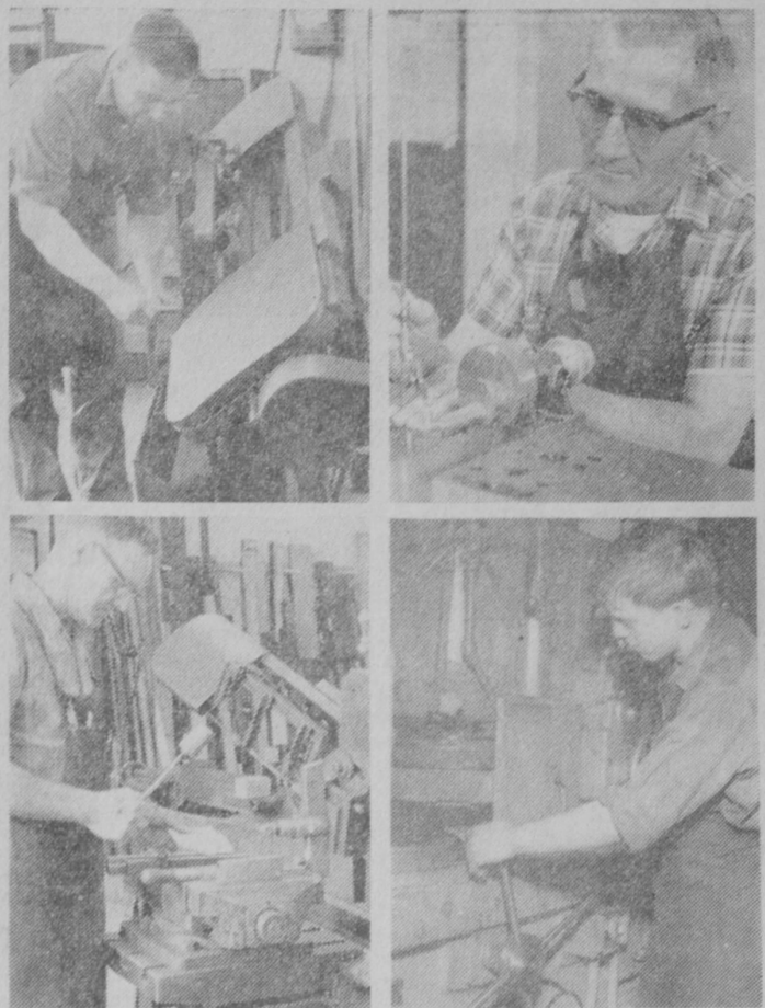
THE FOUR PICTURES show different operations in the plant. At top left, Bernard Freehling operates a cut-off saw, while at top right, Jacob Dittenber sets a diamond on a radius dresser. William Creamer operates a shaper at lower left and Frank Creamer watches stock in a surface grinder at right.
