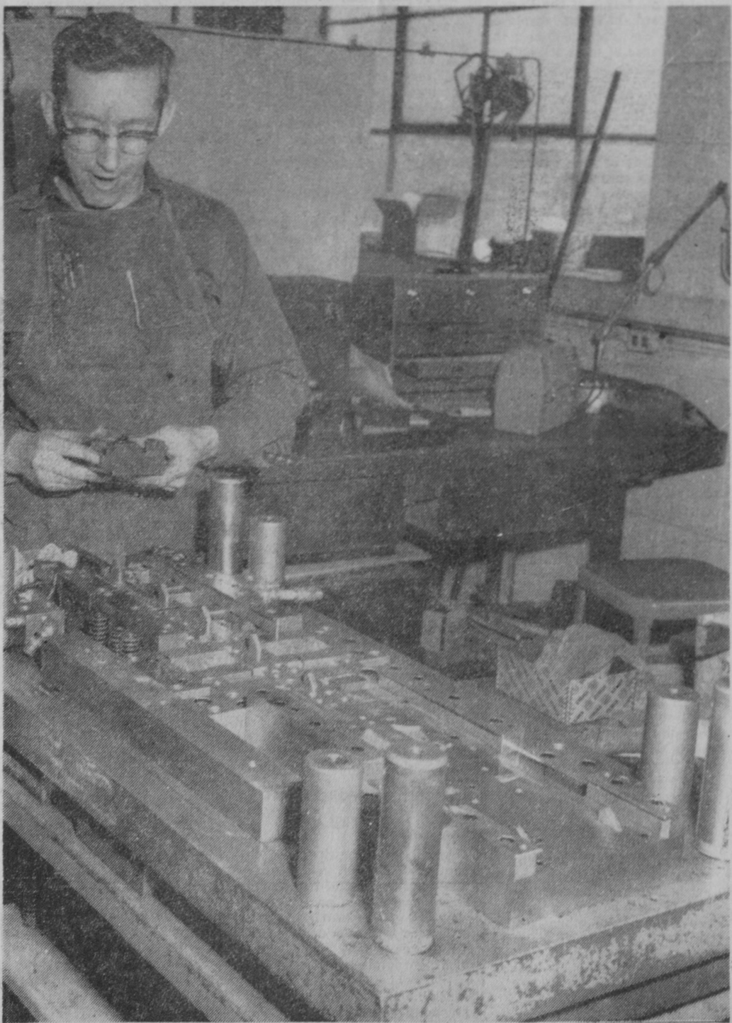
HAROLD CHOLGER is shown here working on one section of a mammoth one-ton die recently constructed at the Tawas City shop. It contains about 150 different operations as it progresses
