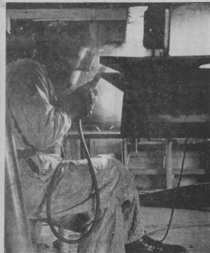
New bolster being welded on frame of car.
