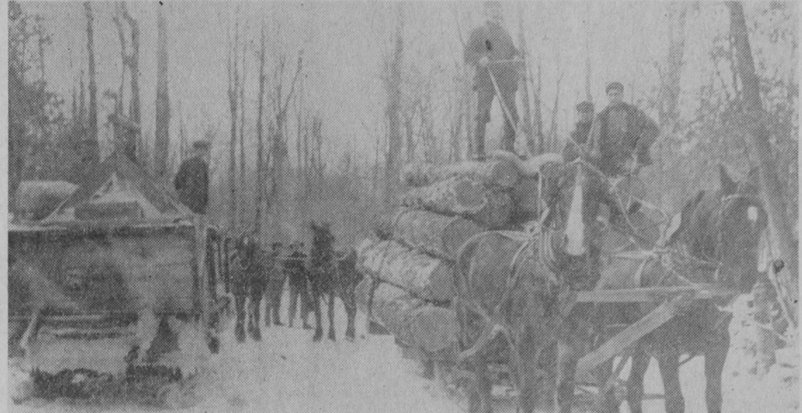
ONE OF THE UNIQUE pictures discovered during Plainfield Township's centennial is the one pictured above. It shows a sleigh loaded with logs at right and a sprinkler at left. The box on the sleigh was filled with water from Hale Creek and drawn over roads at night, sprinkling water as it moved along, to provide a good coating of ice for hauling huge loads.—Tawas Herald Collection.
