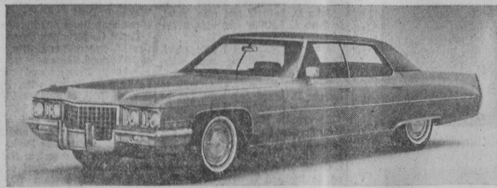
THE 1971 CADILLAC features a new low horizontal front-end motif with widely spaced head lamps set into individual bezels as shown on this Sedan de Ville (top). The front bumper has greater impact and parking protection and enhances the new horizontal look. Two vertical chrome bumper guards with rubber impact strips frame the license plate and reduce possible bumper damage. The grille is of traditional
