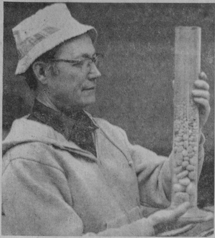
HAROLD FRENCH, chief operator of the water filtration plant at East Tawas, uses a glass tube filled with stones and sand to explain the plant's filtration system.—Tawas Herald Photo.
