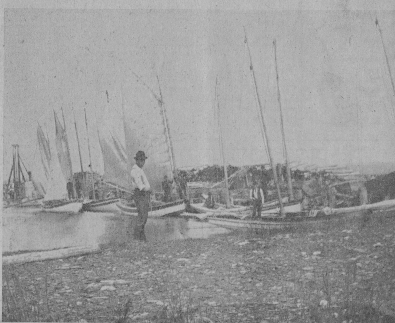
SAILBOATS were used by Saginaw Bay and Lake Huron fishermen for more than one-half century before "one-lung" gasoline engines were installed in boats after 1900. This picture was snapped at East Tawas and shows six sailboats tied up at a dock while the day's catch was being unloaded. At far left is a stake driver used in setting pound or "pond" nets which were used exclusively in
