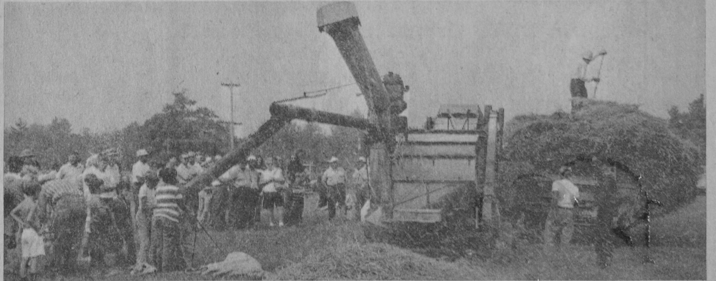
CROUCHING between wagons loaded with grain shocks, the separator gulped down sheaves with a great roaring and shaking and sent out clouds of dust and chaff. Ample power was furnished by
