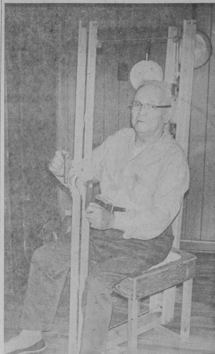
WERNER AHONEN, East Tawas, who observes his 92nd birthday Friday, never got around to patent his invention 20 years ago, but he may do it some day. He developed this back roller to stimulate circulation through manipulation of the spine. The wooden contraption is manually operated and a wooden roller travels the length of the back through use of a pulley arrangement. Ahonen came to the United States from Finland when he was 19 years old and he has been a resident of East Tawas since 1908. He worked for many years with the Superior Fish Company and later as a carpenter, a trade followed by his grandfather in Finland. His wife passed away in April 1976. He makes his home with his daughter, Elsie Solomon, and is to be honored at a family dinner on Friday.—Tawas Herald Photo.
