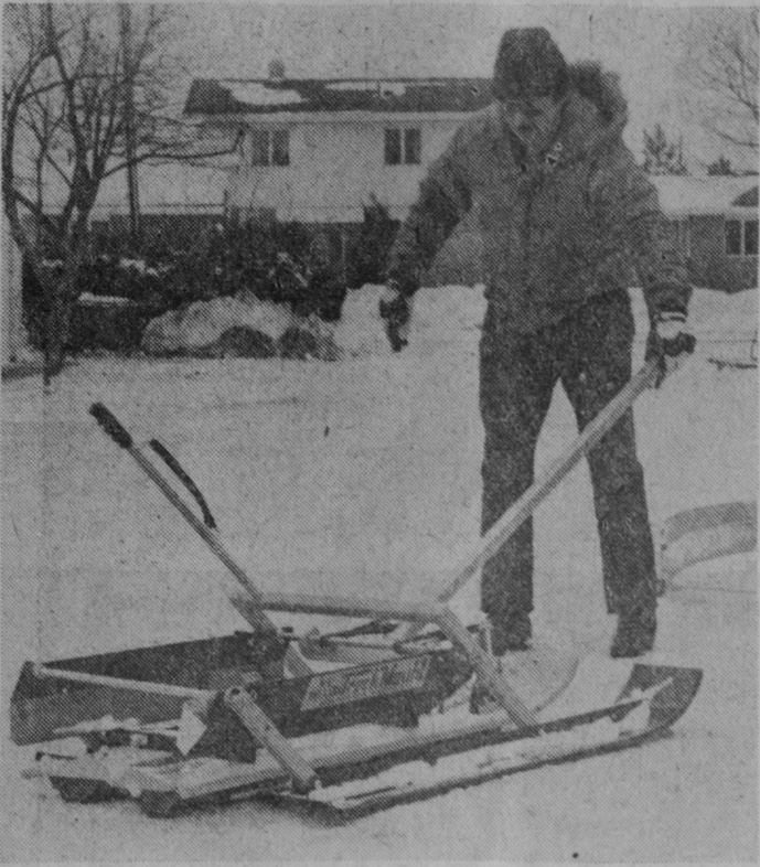
DONALD HOPPE of the United States Forestry Department's Tawas Ranger District demonstrates a new trail groomer which was received for use on cross country ski trails in this area. The unit is towed by a snowmobile and compacts snow into twin tracks in order to improve skiing conditions. Hoppe said the unit would be useful next winter in preparing trails.—Tawas Herald Photo
