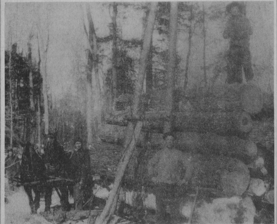
ONE METHOD of loading logs on sleighs was the "horse jammer," pictured here at the Hayes Camp near the AuSable River. A chain passing
