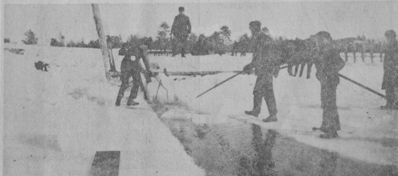
ICE HAS BEEN CUT into large, uniform chunks and the men are using pike poles to move the chunks into position for removal from the water through the use of a team of horses
